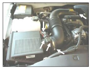
1. **Disconnect the negative battery cable.** Disconnect the Mass Air Flow (M.A.F.) sensor wiring harness. Using the supplied T-20 Security bit, remove the two screws and the M.A.F. sensor from the tube (save the sensor for reuse). Loosen the hose clamps on each end of the factory intake tube assembly.
