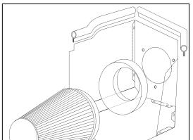
**4.** Using a 10mm socket, remove the five bolts and mounting plate from the engine compartment.
