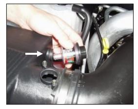
2. Remove the factory filter minder and grommet.
