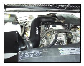
**12.** Install the Airaid intake tube assembly onto the engine. Install the hump hose end onto the filter adapter first and then slip the coupler end of the tube onto the aluminum intake tube. Adjust for fit, and tighten the hose clamps. (*Note: There should be a gap in between the Airaid intake tube and the air filter adapter.*)
