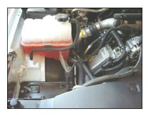
**3.** Remove the factory intake tube assembly from the engine. Rock the factory air box back and forth and remove it from the vehicle. There are only grommets holding it in, no bolts.
