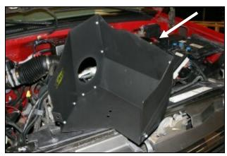
**3.** Assemble the three Cold Air Dam (CAD) panels (#s 2, 3, &4) as shown using nine 6-32 screws (#8), nine #6 washers (#7), and nine nuts (#9).
