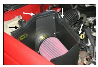
**9.** Install the Airaid Premium Filter (#1) onto the Airaid intake tube as shown, and then tighten the hose clamp. Next, install the weather strip on top of the **CAD**, starting at the right fender working your way towards the front of the vehicle.
