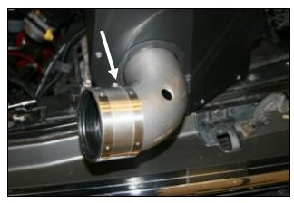
**6.** Install the stainless steel coupler removed in step #1 onto the air intake tube and tighten *only* the hose clamp on the tube.
