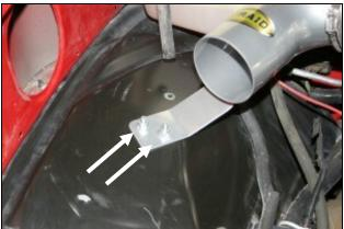
2. Remove the two nuts and washers from the bolts that secure the air intake tube to the inner fender. Save the 3" x 2" plate from the bottom of the fender for reinstallation in step #7. Remove the intake tube from the vehicle.
