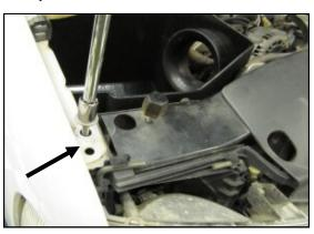
**7.** Using a 13mm socket, remove the factory fender bolt and set it aside. It will be reused in step 8.
