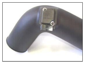
9. Using two 8-32 x 1/2" button head screws (#10) install the factory M.A.F. sensor in the Airaid intake tube (#2) DO NOT USE THE FACTORY SCREWS!
