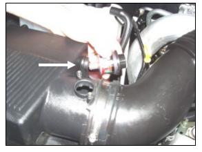
**2.** Remove the factory filter minder and grommet from the side of the factory airbox (save for re-
