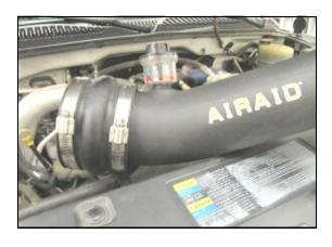
11. Install the urethane hump hose (#5) and two #72 hose clamps (#12) onto the large end of the Airaid Intake tube. (Note: Leave hose clamps loose until final assembly.)
