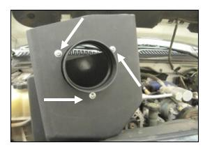
**5.** Install the Filter Adapter (#4) onto the Cold Air **B**ox, or **CAB** (#3), as shown using the three 1/4 -20 Button Head Bolts (#8) and 1/4" Washers (#9).
