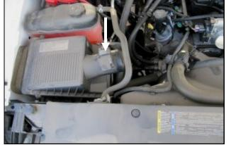
5. Disconnect the Mass Air Flow or MAF sensor and
