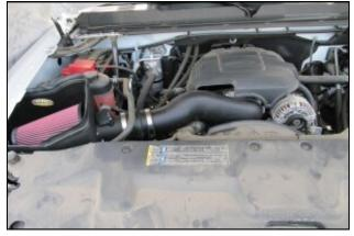
**15.**Reinstall the engine cover. **Double check your work!** Make sure there is no foreign material in the intake path. Make sure all clamps, hoses, bolts, and screws are tight. Double check the hood clearance.
