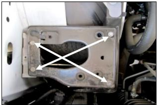
6. Remove the four tray bolts and the airbox mounting
