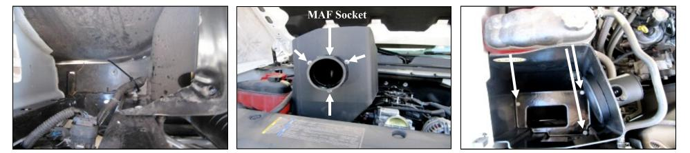
**7.** Secure the wiring harness to the inner fender as shown using the Edge Clip Cable Tie (#14).
