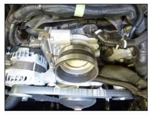
17. Install the appropriate coupler onto the throttle body, The 5.3L engine will use the smaller coupler and the 6.2L engine will use the larger coupler. Secure with the provided hose clamps.
