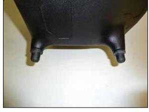
12. Remove the two factory mounting grommets from the factory air filter housing and install them onto the AIRAID® air filter housing.
