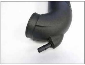
20. Install the grommet and quick disconnect vent fitting into the AIRAID® intake tube as shown.
