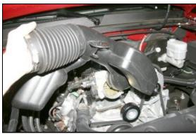
**5.** Slide the factory intake tube off of the **MAF** sensor, rotate it up so that it disengages from the mounting grommet on the intake manifold, and then slide it forward off of the throttle body and
