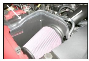
**15.** Install the Airaid Premium Filter (#1) onto the air filter adapter, and tighten the hose clamp. Next install the provided weather strip (#9) onto the top of the **CAD**. For ease of install, start at the inner fender, and work your way towards the radiator. Reinstall the beauty cover.
