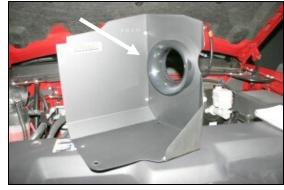
9. Assemble the Cool Air Dam panels (CAD) (#2 & #3) using five 6-32 x 5/16" screws (#10), #6 flat washers (#11), and 6-32 keps nuts (#12). Next install the air filter adapter (#5) into the panels as shown using three 1/4 -  $20 \times 1/2$ " button head bolts (#13), and 1/4" flat washers (#14).
