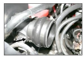
**12.** Install the urethane hump hose (#6), and two #64 hose clamps (#16) onto the **MAF** sensor as shown. Tighten only the clamp on the **MAF** sensor at this time.
