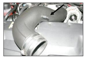
**13.** Install the 1/4" NPT x 3/8" Barb Fitting (#17) into the Airaid Intake Tube as shown. Next install the urethane coupler (#7) onto the throttle body end of the tube using two #64 hose clamps (#16). Tighten *only* the clamp on the tube.
