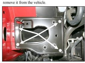
**8.**Using a 10mm socket, remove four bolts, and then remove the factory airbox mounting plate from the vehicle.
