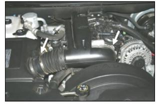
**2.** Using a 5/16" socket or flat blade screwdriver, loosen the hose clamps on both ends of the factory intake tube.
