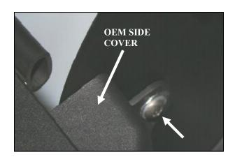
7. <u>6.0 Liter Only:</u> Insert one  $\frac{1}{4}$  - 20 x  $\frac{1}{2}$ " button head bolt (#8) and  $\frac{1}{4}$ " flat washer (#9) through the hole in the oem side cover, and through the hole in the panel. Secure using one  $\frac{1}{4}$  - 20 serrated nut (#10).
