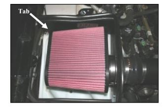
**13.** Install the Airaid Premium Filter (#1) onto the **MAF** sensor. Rotate the filter so that the tab contacts the air box base, and then tighten the clamp. Install the weather strip (#6) onto the top of the panel. (Hint: Start at one end and work towards the other.)
