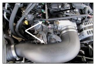
**13. A)** Install the 3/8" Breather Hose (#7) onto the Barbed Fitting and factory hard line.
