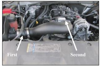
**12.** Install the Airaid Intake Tube assembly onto the Filter Adapter first, and then onto the throttlebody. Adjust for fit, and tighten all hose clamps. Reinstall the hose anchor into the Airaid Intake Tube.
