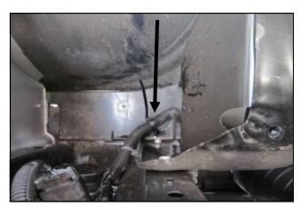
**7.** Secure the wiring harness to the inner fender as shown using the Edge Clip Cable Tie (#14).
