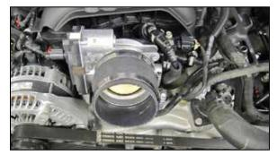
13. Install the coupling hose (08698 for 5.3L, 08497 for 6.2L) to the throttle body and secure with the provided hose clamp.
