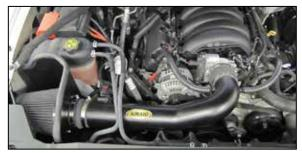
**21. Double check your work!** Make sure there is no foreign material in the intake path. Make sure all clamps, hoses, bolts, and screws are tight. Double check the hood clearance! **Reconnect the negative battery cable!**
