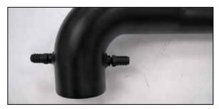
17. Install the two provided crank case vent fittings into the AIRAID intake tube as shown.
