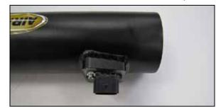
16. Install the mass air sensor into the AIRAID intake tube and secure with the provided hardware.
