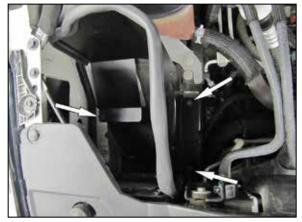
9. Install the heat shield assembly and secure to the air box mounting plate location using the three factory bolts from step #7.
