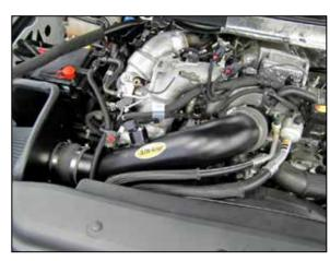
13. Install the intake tube into the coupler installed onto the filter adapter and then into the coupler installed onto the filter inlet. Adjust the tube for best fit and then secure with the provided hose clamps.
