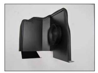
7. Install the provided edge trim onto the heat shield. NOTE: Some trimming of the edge trim will be necessary.
