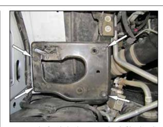
5. Remove the four bolts that secure the air filter housing mounting plate to the inner fender and then remove the mounting plate from the vehicle.
