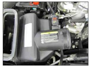
4. Release the red locking tab and then disconnect the mass air sensor electrical connection. Unhook the coolant bypass hose from the air filter housing. Lift the air filter housing up to dislodge it from the mounting grommets and remove it from the vehicle.
