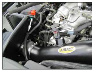
14. Reconnect the mass air sensor electrical connection and secure the coolant bypass hose to the heat shield using the factory retaining clip.
