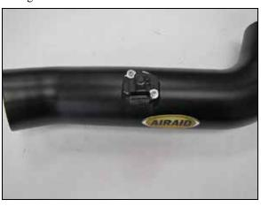
12. Install the mass air sensor into the AIRAID intake tube and secure with the provided hardware.
