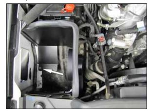
8. Install the heat shield assembly into the vehicle and secure it to the inner fender with one of the factory bolts from step #5 where shown.
