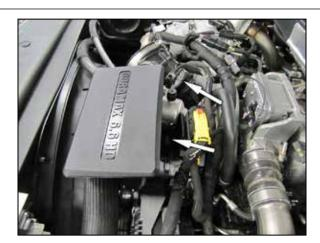
3. Remove the nut that secures the intake plenum to the Engine and then loosen the hose clamp that secures the plenum to the turbo inlet. Remove the intake plenum from the vehicle.
