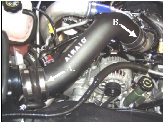
13. A.) Install the hump hose end of the Airaid intake tube assembly onto the filter adapter first. B.) Slip the coupler end of the tube over the factory turbocharger inlet. Adjust for fit, and tighten the hose clamps. (Note: There should be a gap in between the Airaid intake tube and the air filter adapter.)
