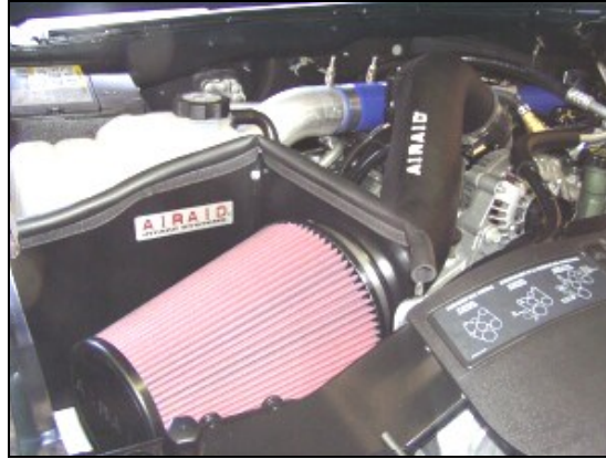
14. Install the Airaid Premium Filter (#1) onto the filter adapter, and tighten the hose clamp. Install the weather strip (#8) onto the Airaid Cool Air Dam. Reconnect the M.A.F. sensor wiring harness. (Note: Start from one corner and work your way around to insure proper alignment of the weather strip.)
