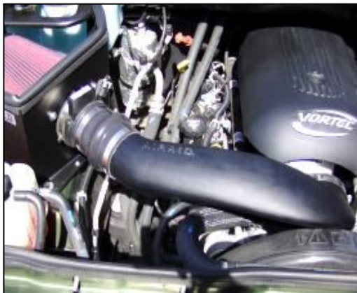
13. Connect the Airaid MIT (#5), hump hose end first, to the MAF sensor, and then connect the other end of the tube assembly to the throttle body. Check for interference and adjust the MIT accordingly, and then tighten the hose
