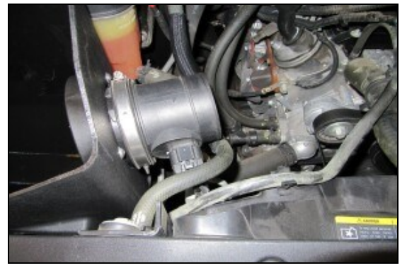
12. Reinstall the MAF sensor onto the Filter Adapter, and tighten the clamp.
