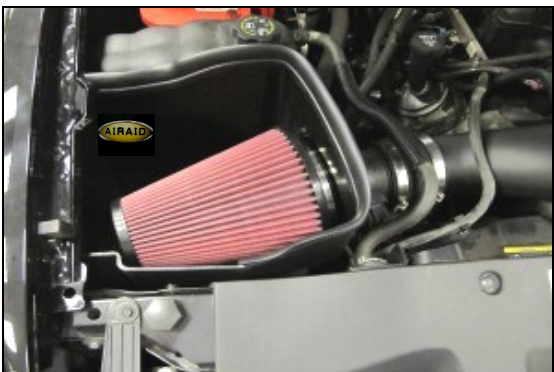
13. Install the Airaid Premium Filter (#1) onto the Air Filter Adapter, and tighten the hose clamp. Next install the provided Weather Strip (#8) onto the top of the CAB. For ease of install, start at the inner fender, and work your way towards the radiator. Reinstall the engine cover.
