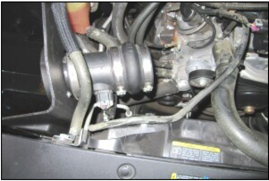
13. Install the Urethane Hump Hose (#5), and two #64 Hose Camps (#11) onto the MAF sensor as shown. Tighten only the clamp on the MAF sensor at this time.
