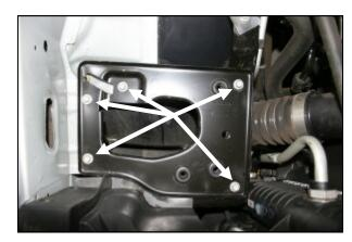
**3.** Using a 10mm socket, remove 5 bolts, and then remove the factory air filter mounting plate.
