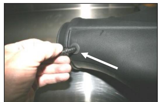
6. Install the provided grommet (#13) into the hole in the Airaid Intake Tube (#2). Next install the factory plastic breather fitting removed in step #5 into the grommet.
