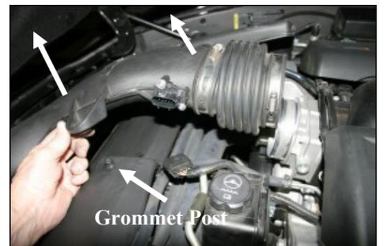
3. Lift up on the factory intake tube assembly to disengage the grommets from the three grommet posts and throttle body. Remove the assembly from the vehicle.
