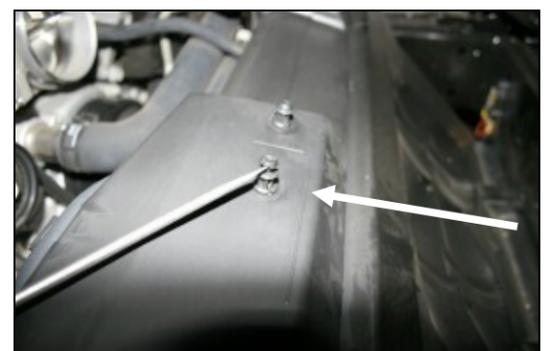
9. Using a flat blade screwdriver, pry up the center pin in the grommet post closest to the right fender on the radiator shroud, and remove both pieces of the grommet post from the vehicle.
