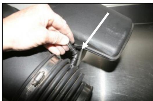
5. Remove the factory breather fitting from the factory intake tube and save it for reinstallation in step #6.
