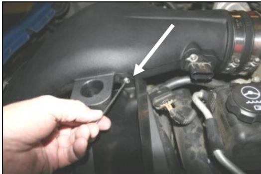
14. Tighten all four button head bolts that secure the air dams to the intake tube, and the radiator shroud.
