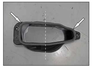
10. Install the foam gaskets onto the AIRAID® air filter housing in the location shown. **NOTE: Be sure the area the gasket applies is clean before installing the gaskets.**
