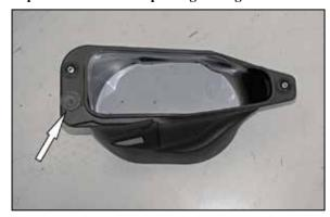
9. Transfer the factory air filter housing mounting grommet to the AIRAID® air filter housing in the location shown.
