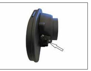
12. Remove the mass air sensor from the factory housing and then install it into the AIRAID® housing and secure with the provided hardware.
