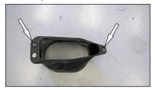
8. Insert the mounting grommets with sleeves into the AIRAID® air filter housing at the two locations shown. NOTE: The rubber grommets will be on both sides of the part with the sleeve passing through them.
