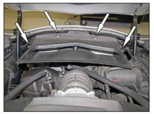
2. Remove the four screws that secure the radiator heat extractor duct to the radiator and then remove the duct from the vehicle.
