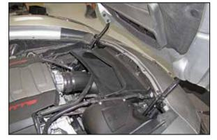
26. Reinstall the radiator heat extractor duct and secure with the factory hardware.
