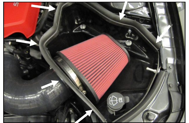
18. Install the Airaid Premium Filter (#1) onto the filter adapter and tighten the clamp. Next install the weather strip onto the top of the CAB. For ease of installation, start the front of the CAB near the radiator and work your way around towards the fender. Re connect the negative battery cable.
