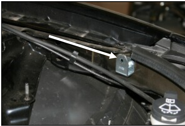
11. Install the side bracket (#12) onto the inner fender as shown using the 6mmx12mm hex bolt (#15), and lock washer (#14).
