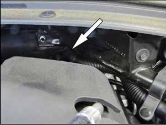
8. At the firewall, Remove the 6mm flange nut that secures the sound tube to the firewall. Turn the tube ¼ turn clockwise and the remove the tube from the vehicle.
