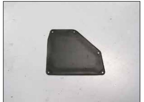
21. Install the provided gasket onto the air filter housing lid.
