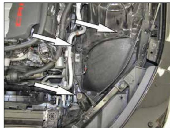
5. Be sure that all three mounting grommets are still in the proper place and not still attached the factory air filter housing.
