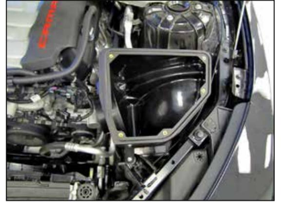
17. Install the AIRAID filter housing into the vehicle so that the mounting posts are engaged into the factory filter housing mounting grommets.
