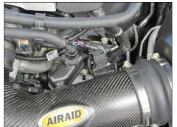
19. Connect the crank case vent hose to the PCV vent chamber and connect the mass air sensor electrical connection.
