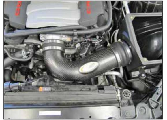
18. Install the coupler houses and hose clamps onto the AIRAID intake tube but do not tighten the clamps. Install the intake tube assembly onto the filter adapter and throttle body. Adjust the assembly for best fit and then secure all the hose clamps.
