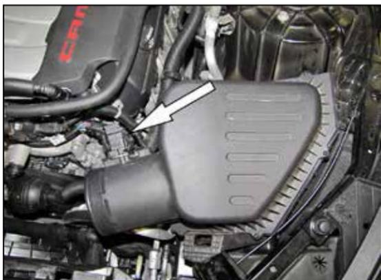
4. Disconnect Mass air flow sensor electrical connection and then lift and remove the complete air filter housing from the vehicle. **NOTE: Airaid recommends that customers do not discard factory air intake.**
