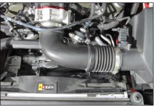
7. Reinstall the intake tube, tighten the two hose clamps, and reconnect the crankcase breather tubes. Reinstall the beauty cover, and oil cap in the reverse order in which they were removed.
