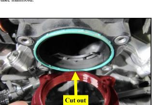
**5.** Install the Spacer <u>into</u> the intake manifold as shown with the cut out in the 6 O Clock position. When properly installed, the Spacer sleeve will be inside the manifold and the flange will be flush.
