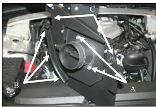
**9. A)** Transfer the Mass Air Flow Sensor from the factory airbox to the Adapter Panel and secure using two 1/4-20 button Head Screws (#15) and Serrated Nuts (#17). Note: The factory airbox seal on the Mass Air Flow Meter is not to be used in this kit. **B)** Attach the Weather Strip (# 11) to the curved edge of the MAF Panel. **C)** Insert the 5/8" hose anchors (#28) into the two horizontal tab holes on the MAF panel.
