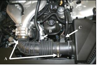
**2. A)** Loosen the hose clamps on the factory intake tube. **B)** Disconnect the breather line and remove the factory intake tube . **C)** Disconnect the Mass Air Flow sensor.
