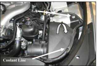
**3. A)** Remove the factory fender bolt securing the air box assembly. Next pull out the coolant line from atop the air box lid and gently rotate the air box assembly towards the front of the vehicle. The air box assembly is now free and should be removed from vehicle.
