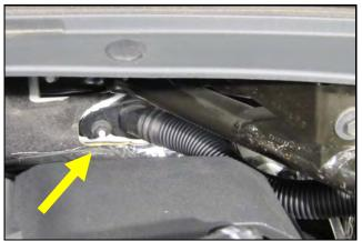
**6.** At the firewall, remove the 6mm flange nut at the resonator tube base. Turn the tube 1/4 turn Clockwise and remove the entire resonator from the vehicle. It will not be reused.
