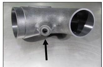
**9.** Insert the grommet into the Intake Tube as shown.
