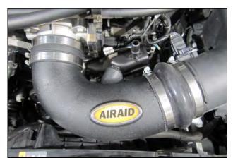
**13.** Insert the Intake Tube into the coupler first, then into the Hump Hose. Tighten all four clamps at this time.
