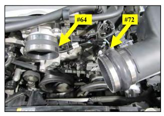
**12.** Slide the Coupler and the 64 Clamps onto the throttle body and the Hump Hose with the 72 Clamps onto the airbox outlet.
