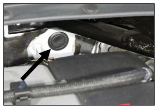
7. Insert the Firewall Plug into the resonator tube hole.
