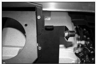
**8.** Attach the 5/8" Well Nut (#22) to the vertical MAF Panel tab as shown using the 5/16 Hex Bolt (#20) and the 5/16" flat washer (#21).
