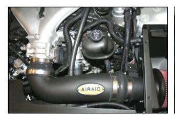
**13.A)** Install the Airaid Intake Tube assembly onto the Mass Air Flow Sensor first, and then onto the throttle body. Adjust for fit, and tighten the hose clamps. **B)** Replace the factory breather line on the valve cover with the 26" Airaid Breather Hose(#11). Secure the breather hose to the intake tube nipple using the black Speed Clamp (#29)
