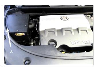
**12**. **A)** Attach the Weather Strip (#7) to the curved edge of the Top Panel (#5). **B)** Attach the Top Panel to the Airaid Performance Airbox using the four 1/4-20 Phillips Head Screws. Reinstall the engine cover and the oil fill cap.
