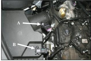
**3.** Disconnect the Mass Air Flow, or MAF sensor (A) and the MAP sensor (B) from the factory airbox lid.
