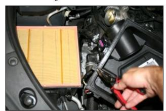
**4.**Turn the factory airbox lid over and locate the wire harness anchor. Using a pair of needle nose pillars, compress the ribs of the anchor and remove it. Remove the factory air filter and set it aside.
