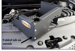
tabs on the **outside**, using the four 6-32 screws (#15), #6 Flat washers (#14), and #6 Keps Nuts (#13).
