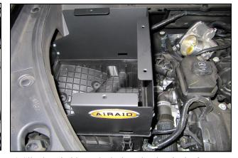
6. Slip the Airaid Panel tabs into the slots in the factory airbox and partially install the Panel assembly onto lower half of the factory airbox as shown. Do not latch the airbox clips at this time.
