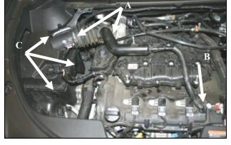
**2. A)** Loosen the hose clamps on the factory intake tube. **B)** Disconnect the crank case breather line at the valve cover, and remove the factory intake tube. **C)** Unfasten the 3 Factory air box clips.
