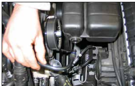
4. Disconnect the crank case vent tube from the intake resonator as shown.
