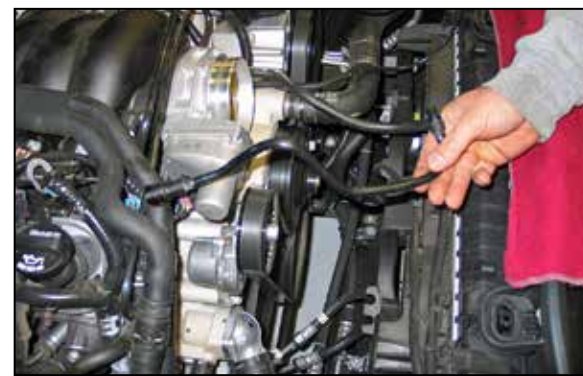
6. Rotate the crank case vent tube 180°, then release the retainer at the valve cover port and then remove the crank case vent tube.
