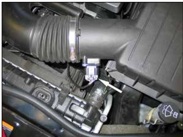
2. Disconnect the mass air sensor electrical connection.
