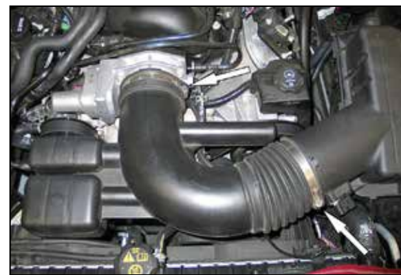
5. Loosen the hose clamps which secure the stock intake tube to the air box and throttle body and then remove the stock intake tube from the vehicle.
