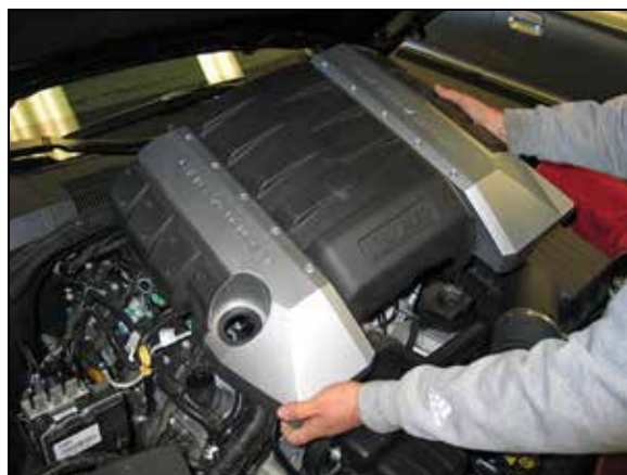
3. Remove the oil filler cap and then lift up and remove the engine cover. Reinstall the oil filler cap.
