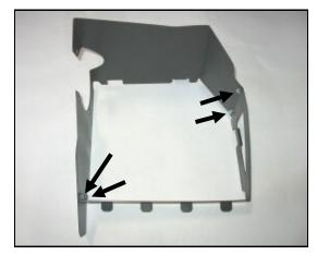
9. Assemble the Airaid Cool Air Dam (CAD) panels (#2,#3) using four 6-32x 5/16" screws (#7), #6 flat washers (#8) and 6/32 keps nuts
