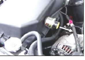
**3.** Using a 7mm socket, loosen the hose clamp where the factory intake tube connects to the turbo housing.
