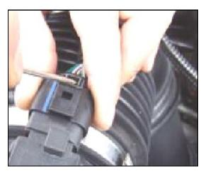
**14.** Reconnect the **IAT** sensor wiring harness to the sensor.
