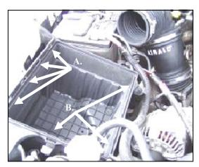
**12.** A.) Install the **CAD** by inserting the four tabs into the side of the factory airbox.
