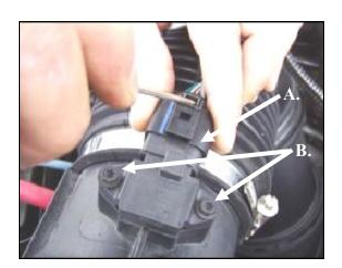
1. Disconnect the negative battery cable. A.) Disconnect the Intake Air Temperature (IAT) sensor wiring harness by pushing down on the tab, and sliding the connector back. **B**.) Using the provided T-20 torx bit, remove the two IAT sensor mounting bolts and the sensor from the tube (save for reuse).
