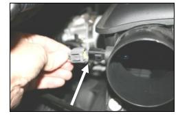
3. Squeeze the tab on the connector, and disconnect the air intake temperature sensor on the back of the resonator.
