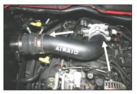
11. Install the Modular Intake Tube (#3) into the hump hose first and then into the factory coupler. Adjust for fit, and then tighten all 3 hose clamps.
