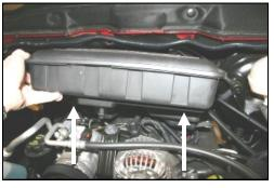
5. Lift the front of the resonator straight up, and then pull towards you to remove it from the vehicle.
