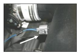
**13.** Re-connect the wiring harness to the factory temperature sensor on the back of the Modular Intake Tube (#3).
