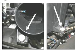
4. With a 10mm socket, remove two bolts holding the intake resonator to the intake manifold brackets.
