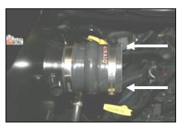
7. Install the supplied grommet (#10) into the Modular Intake Tube (#3). Next, carefully slide the factory temperature sensor into the grommet until it touches the tab on the temperature sensor.
