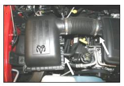
Disconnect the negative battery cable! Loosen the hose clamp on the resonator. Disconnect the breather hose going into the factory airbox lid.
