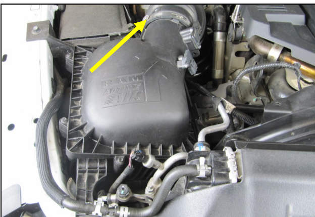
3. Loosen the clamp on the intake tube and remove the airbox lid from the vehicle.
