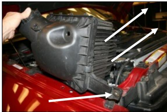
**2.** Using a 10mm socket, remove the nut that secures the factory airbox to the radiator support. Next slide the flexible intake tube off of the factory airbox lid and then rock the factory airbox assembly side to side to release it from the mounting grommets, and remove it from the vehicle.
