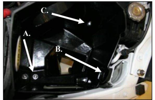
**9.** Install the CAB into the vehicle as shown. **A.)** Install the 3/8" button head bolt (#17) and flat washer (#18) thru the CAB and into the well nut. **B.)** Install the M6 x 25mm hex bolt (#15) and flat washer (#10) thru the CAB and into the captured nut in the fender. **C.)** Install the 5/16" bolt (#11) flat washer (#12), and flange nut (#13) thru the CAB and L-bracket. Tighten all mounting bolts at this time.
