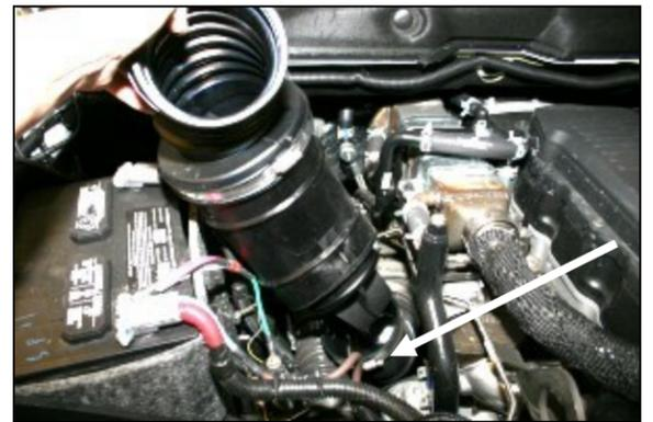
**3.** Loosen the hose clamp that secures the factory intake tube assembly to the rubber elbow on the turbo inlet, and remove the assembly from the vehicle.
