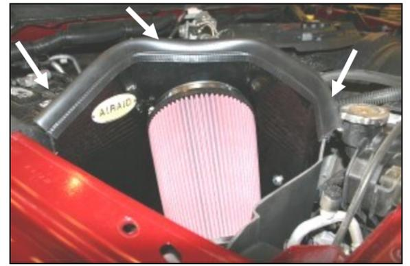
12. Install the Airaid Premium Filter (#1) onto the filter adapter and tighten the clamp. Install the weather strip onto the top of the CAB starting at the right fender and working your way towards the radiator.
