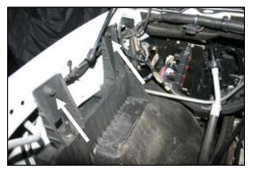
**9.** Remove the two bolts that secure the factory airbox mounting bracket to the inner fender. They will be reinstalled in step #10.
