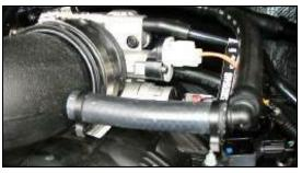
15. 2002-03 Models: Install one end of the provided 90° barbed fitting (#22) into the factory breather hose and then connect the supplied 1/2" breather hose (#21) to the other end. Connect the hose to the nipple on the Airaid intake tube. Secure all three connections with the provided #16 Speed Clamps (#17).
