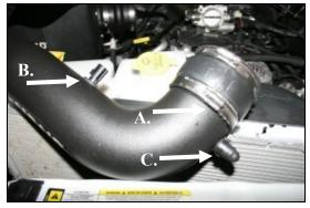
12. 2002-07 Models: A.) Reinstall the factory coupler and hose clamps on to the Airaid intake tube (#2). (2008-12 Models: use the supplied coupler (#5), and #48 hose clamps (#10). Tighten the hose clamp on the tube.
