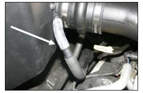
14. 2004-12 Models: Reconnect the factory breather hose to the 1/2" barbed fitting on the CAB using the 1/2" rubber elbow (#15), and 1/2"x 3/4" barbed fitting (#20) as shown.
