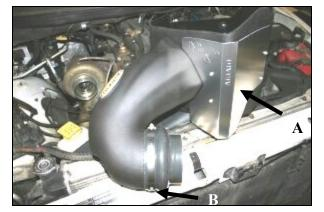
5. A) Install the aluminum Heat Shield (#4) onto the CAB using the four 1/4" Button head Bolts (#7) and the Flat washers (#8). Remove the protective film from Heat Shield. **B)** Install the silicone reducer (#5) on to the Airaid Intake Tube (#2) using the #80 (#14)
