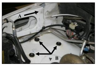
6. A) Remove the Factory 8mm fender bolt and set aside, it will be reused later in step 8. B) Place the 1/4" I.D. Grommets (#12) over each of the three studs on the inner fender.
