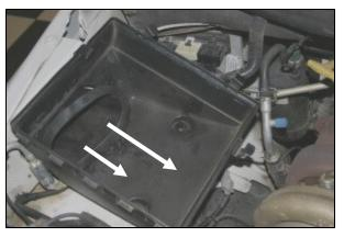
3. Locate the fender air scoop inside of the factory air box and remove it by pulling outward. The remaining factory airbox half can now be removed by simply pulling upward and off of the mounting studs on the inner fender well.
