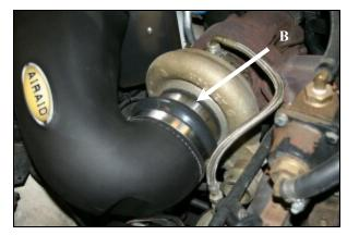
7. A) Install the CAB and Tube assembly onto the turbo inlet first, then rotate the assembly downward onto the inner fender studs. B) Secure the Silicone reducer to the turbo inlet using the # 64 Clamp (#13). C) Fully tighten the three 1/4" Button Head Bolts from step 4.
