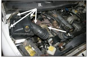
1. Disconnect the negative battery cables. A) Loosen the hose clamp on the factory turbo inlet tube. B) Unfasten the Four clips on the right, left, and back side of the airbox. Remove the airbox lid and tube as an assembly and set aside.
