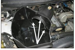
4. Attach the Intake Tube (#2) to the Cool Air Box, (CAB) (#3) using three 1/4" Button Head Bolts (#7) and Flat Washers (#8) as shown. Do not fully tighten the bolts at this time.
