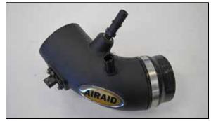
13. Install the provided step coupler onto the AIRAID intake tube as shown.
