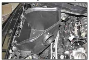
10. Install the AIRAID filter housing onto the factory air filter housing mounting studs and secure with the hardware provided.
