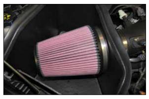
17. Install the air filter onto the filter adapter and secure with the provided hardware.
