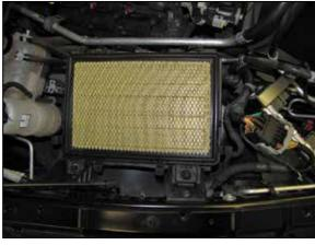
5. Lift the lower air filter housing up and then remove the housing from the vehicle.
