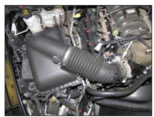
4. Loosen the hose clamp that secures the factory intake tube to the throttle body, release the four clips that secure the upper air filter housing and then remove the upper air filter housing and intake tube from the vehicle.
