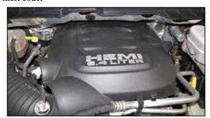
2. Lift the decorative engine cover up and remove it from the vehicle.
