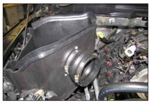
14. Install the provided hump coupler onto the filter adapter as shown.
