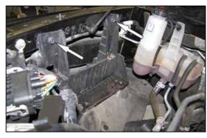
6. Remove the two upper filter housing bracket mounting bolts.
