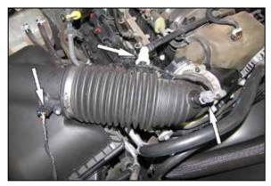
3. Disconnect the mass air sensor and inlet air temperature sensor electrical connections and disconnect the crank case vent quick connect fitting.
