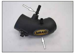
12. Install the provided quick connect vent fitting and AIRAID decal onto the AIRAID intake tube as shown. NOTE: Plastic NPT fittings are easy to cross thread. Install the vent fitting "hand" tight, then turn it two complete turns with a wrench.
