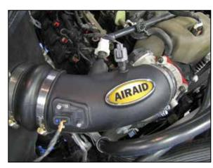
16. Connect the crank case vent to the fitting installed into the AIRAID intake tube. Reconnect the mass air sensor and inlet air temperature sensor electrical connections.
