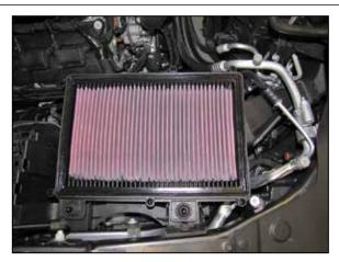
5. Install the AIRAID<sup>®</sup> air filter and then replace the factory lid and secure with the factory screws.
