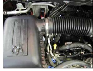
4. Loosen the hose clamp securing the intake hose to the factory air box.
