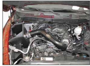
**26. Double check your work!** Make sure there is no foreign material in the intake path. Make sure all clamps, hoses, bolts, and screws are tight.
