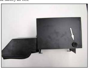
11. Install the factory rubber mounting grommet into the AIRAID heat shield as shown.
