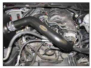
22. Install the intake tube assembly into the coupler hose at the filter adapter and then into the coupler hose at the throttle body. Adjust the tube for best fit and then secure with the provided hose clamps.
