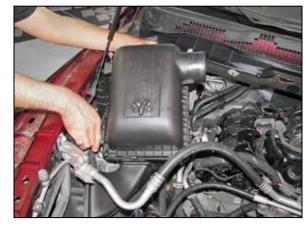
6. Lift the air box assembly off of the mounting studs and then remove the air box from the vehicle. NOTE: AIRAID recommends that customers do not discard factory air intake.
