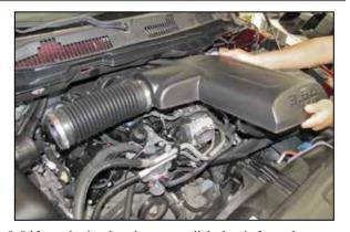
5. Lift up the intake plenum to dislodge it from the mounting grommets and then remove the plenum from the vehicle.
