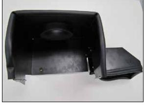
12. Install the air filter adapter into the heat shield and secure with the provided hardware.
