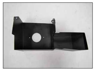
7. Install the fresh air intake scoop onto the heat shield and secure with the provided hardware.
