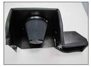
13. Install the air filter onto the filter adapter and secure with the provided hose clamp.
