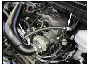
25. Install the crank case vent hose assembly onto the fitting installed into the intake tube and then connect the quick disconnect fitting into the factory connector as shown.
