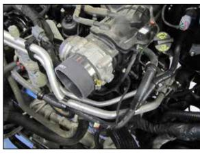
17. Install the provided coupling hose (08690) onto the throttle body and secure with the provided hose clamp.
