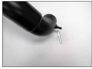
20. Install the inlet air temperature sensor into the grommet installed into the intake tube.
