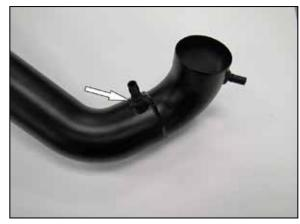
21. Install the provided vent fitting into the intake tube as shown.
