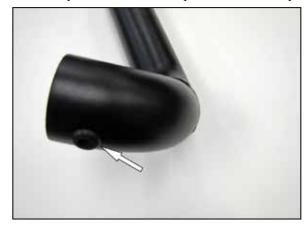
18. Install the provided grommet into the intake tube.
