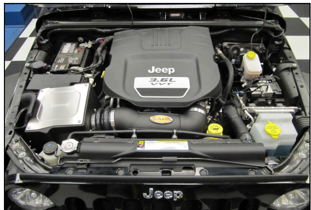
20. Double check your work! Make sure there is no foreign material in the intake path. Make sure all clamps, hoses, bolts, and screws are tight. Double check the hood clearance! Reconnect the negative battery cable!
