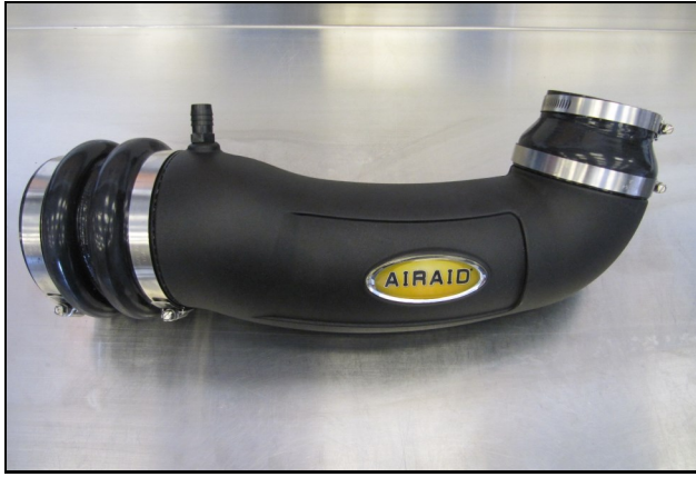
13. Slide the Double Hump Hose (#6), and two #72 Hose Clamps (#28), onto straight end of the Tube. Slide the Silicone Reducer (#7) and the #48 and #64 Clamps on the 90 deg. bend of the Intake tube. Leave the Clamps loose for now.
