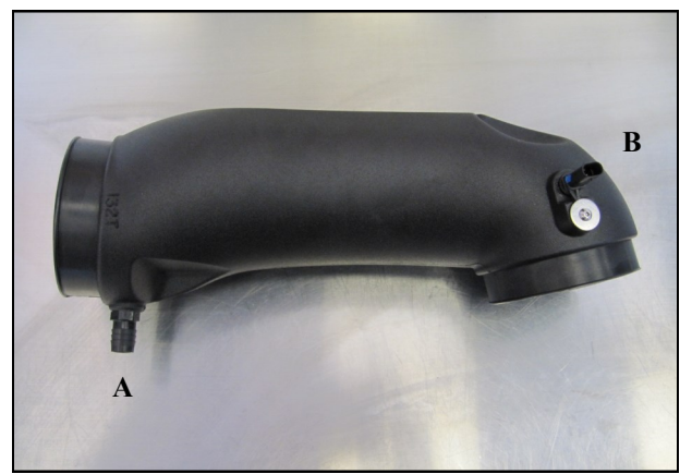
12. A.) Install the 5/8" Barbed Fitting (#24) into the threaded 3/8 hole in the side of the Airaid Intake Tube (#2). B.) Transfer the air temp sensor from the factory intake into the Airaid Intake Tube and secure it using the #8-32 x 1/2" Button Head Bolt (#20) and #8 Fender Washer(#19).
