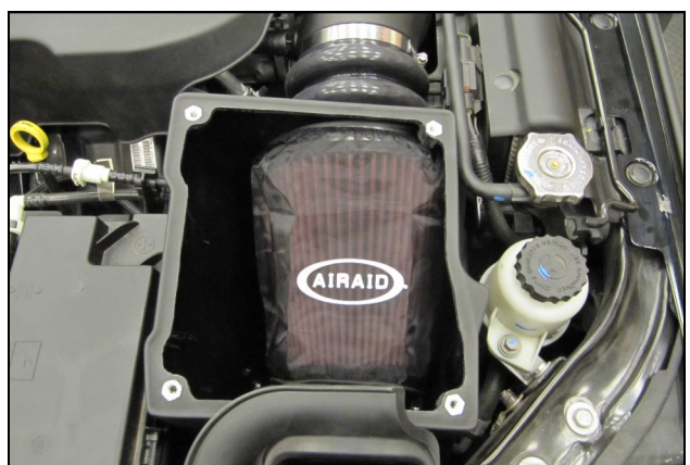
21. Pre Filter Option: Part Number 799-445 For maximum protection in the harshest environments Airaid offers a slip on Pre Filter. - Prolongs Cleaning Intervals - Water Repellant - Free Flowing Protection
