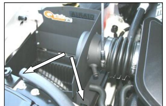
**6.** Install the Quick Fit Panels by sliding the four tabs on the back of the panels into the factory airbox base, and then into the factory intake tube. Relatch the two factory clips into the slots on the front of the Quick Fit Panels. Tighten the hose clamp on the factory intake tube.
