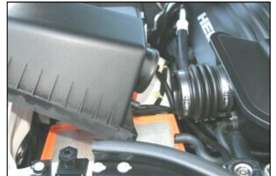
**3.** Remove the factory airbox lid by sliding it forward, and then up and out of the factory intake tube.
