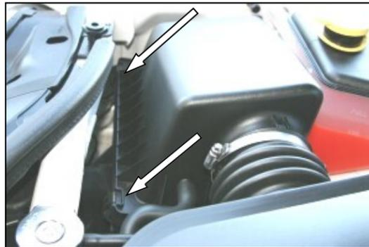
**2.** Unlatch the two clips on the front of the factory airbox lid.
