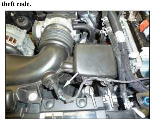
2. Disconnect the inlet air temperature sensor electrical connection and unhook the wiring harness from the intake plenum.
