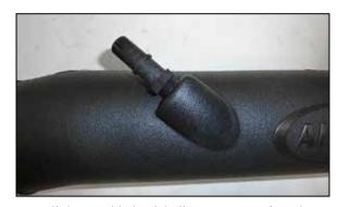
7. Install the provided quick disconnect vent into the AIRAID® intake tube as shown.
