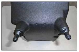
9. Install the two provided mounts onto the bottom of the air filter housing using the provided hardware.
