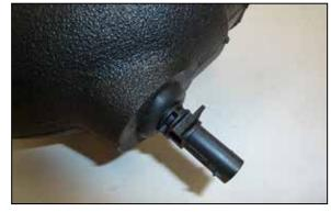
6. Install the provided grommet into the AIRAID® intake tube. Remove the inlet air temperature sensor from the factory intake tube, Remove the O-ring from the sensor and then install the sensor into the grommet installed into the AIRAID® intake tube.
