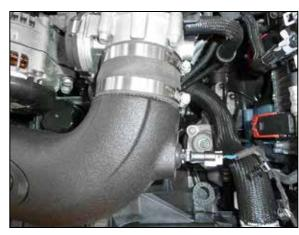
15. Reconnect the inlet air temperature sensor electrical connection.
