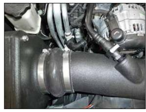
16. Connect the factory crank case vent hose to the quick disconnect fitting installed into the AIRAID® intake tube.
