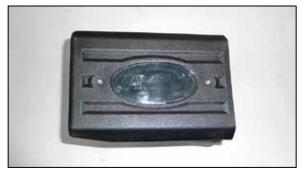
8. Install the AIRAID® window into the air filter housing using the provided hardware.
