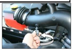
7. Carefully twist and remove the temperature sensor from the stock intake tube. Remove the stock intake tube from the vehicle.
