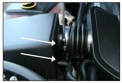
1. Disconnect the negative battery cable. Loosen hose clamp on air cleaner box lid. Carefully twist and remove the breather hose from the lid.
