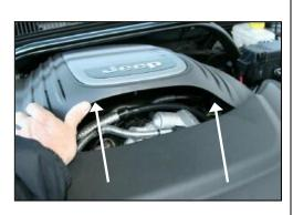
3. Carefully lift the engine cover for access to the throttle body. (There are only grommets that hold down the cover, no bolts.)
