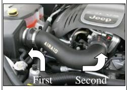
13. Install the MIT into the hump hose first, and then into the throttle body coupler. Adjust to fit, and tighten the hose clamps.
