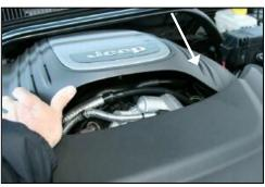
**14.** Re-install the engine cover by firmly pushing it back into the grommets.
