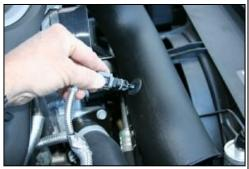
12. Carefully install the temperature sensor into the Airaid MIT as shown. Make sure it's pushed all the way in and the plug is connected to the wire harness.
