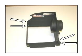
**5.** Assemble the Quick Fit Panels (#2, #3) using four 6-32 x 5/16" screws (#5), #6 flat washers (#6), and 6-32 keps nuts (#7).
