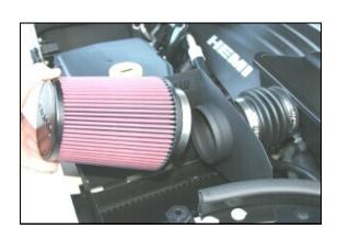
**8.** Install the Airaid Premium Filter (#1) onto the tube on the Quick Fit Panels, and tighten the clamp.
