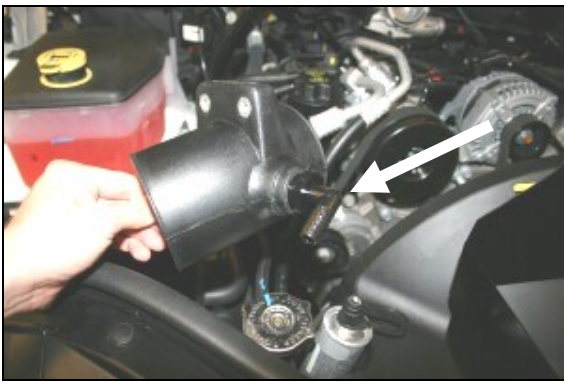
10. Install the 90° nylon fitting (#9), into the air filter adapter.
