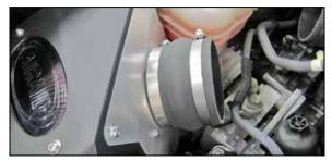
14. Install the provided coupler hose (08418) onto the filter adapter and secure with the provided hose clamp.
