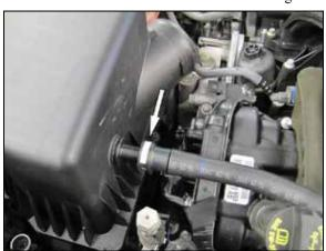
4. Disconnect the crank case quick connect fitting from the factory air filter housing. Pull up firmly on the air filter housing and remove it from the vehicle.
