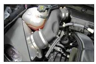
17. Install the intake tube assembly into the coupling hoses, adjust for best fit and then secure with the provided hose clamps.
