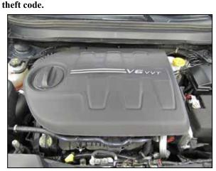
2. Lift up and remove the decorative engine cover to remove it from the engine.
