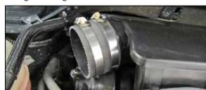
13. Install the provided coupler hose (08690) onto the intake plenum and secure with the provided hose clamps
