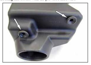
11. Remove the two mounting grommets from the factory air filter housing and install them into the AIRAID air filter housing as shown.
