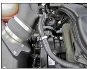
18. Connect the factory crank case quick connect fitting to the quick connect fitting installed onto the AIRAID intake tube.
