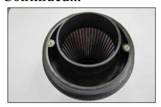
8. Install the radius adapter into the air filter as shown and secure with the provided hose clamp.
