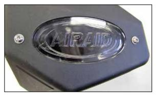
5. Install the AIRAID window into the AIRAID air filter housing using the provided hardware.
