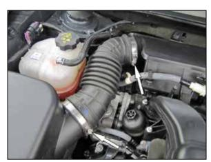
3. Loosen the hose clamps that secure the factory intake tube and then remove the intake tube from the engine.
