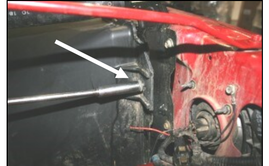
9. Remove one bolt from the passenger side radiator fan shroud and save it for step #15.
