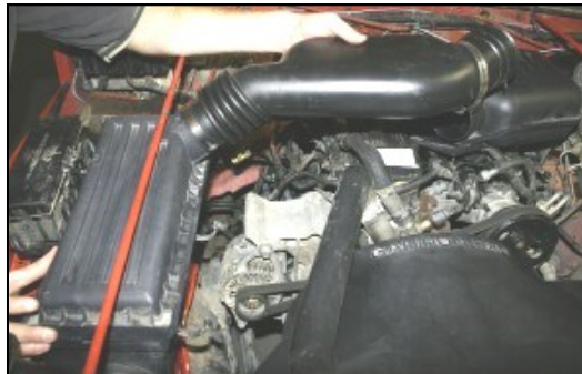
2. Unlatch the clips on the factory air cleaner lid, next remove the lid, and tube as an assembly.
