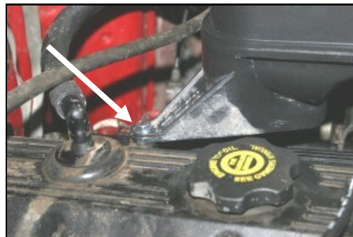
5. Remove the bolt that holds the resonator to the valve cover.
