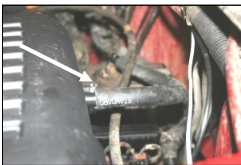
4. Disconnect the breather hose from the resonator.
