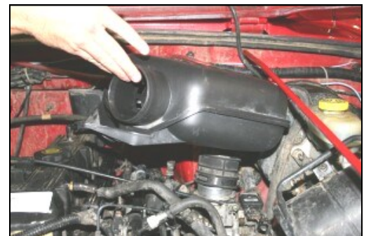
6. Remove the resonator from the vehicle.
