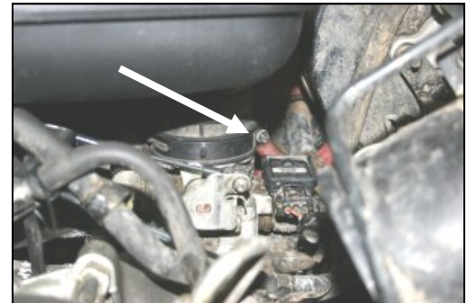
3. Loosen the clamp that holds the resonator to the throttle body.
