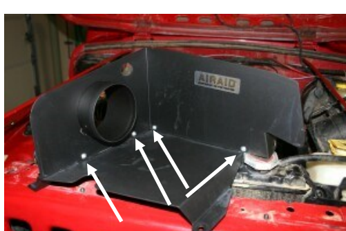
11. Assemble the two Cool Air Dam panels (#2) & (#3) using the four 6-32 screws (#8), #6 flat washers (#9), and nuts (#10), as shown.
