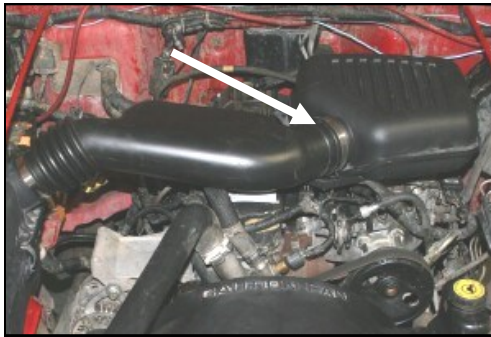
1. Disconnect the negative battery cable. Loosen the hose clamp that holds the factory intake tube to the resonator.
