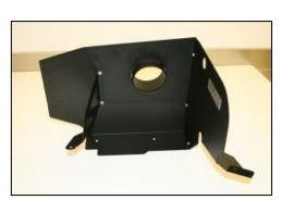
7. Assemble the Cool Air Dam (CAD) panels (#2, #3, & #4) as shown using the 5 provided screws (#10), washers (#11), and nuts (#12).
