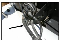
11. Slide the CAD bracket under the horn mount and reinstall the factory bolt from step 5.
