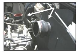
15. Install the urethane hump hose (#6) on the CAD with two #60 hose clamps (#18), and the coupler (#7) on the throttle body with two #44 hose clamps (#17). Leave the clamps loose for now.
