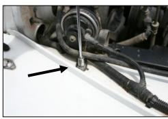
5. Using a 10mm socket, remove the horn bolt from the fender. (Save for later use.)
