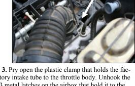
tory intake tube to the throttle body. Unhook the 3 metal latches on the airbox that hold it to the mounting plate, and remove the intake assembly.
