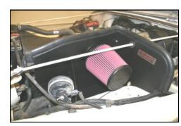
**18.** Install the Airaid Premium Filter (#1) and the weather strip (#9) onto the **CAD**, as shown. (Hint: start the weather strip near the radiator support and work towards the back of the vehicle.)
