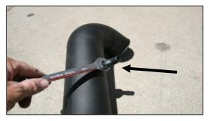
**14.** Install the ½" barbed fitting (#22) into the intake tube.
