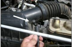
2. Disconnect the vacuum line from the airbox and at the canister below the master cylinder. (Save for reuse.)
