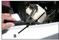
**12.** A) Using a ½-20 bolt (#13), 2 washers (#14), and locknut (#16), bolt the CAD to the fender. B) Install the wire loom clamp into the hole in the **CAD**, as shown.
