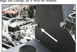
**9.** Carefully slide the **CAD** over the support rod, and then slide the supplied grommet over the rod, and into the hole in the **CAD** as shown. Rotate the CAD and place it into position on the factory airbox mount. Re-install the radiator support rod, and tighten the nut.
