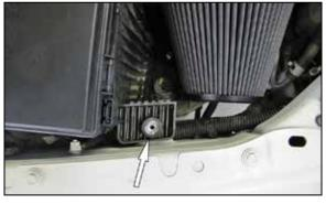
16. Install the rubber mounted stud into the air box mounting plate bolt location as shown.
