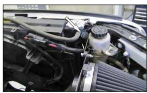
15. Install the heat shield bracket assembly onto the heat shield and radiator mount as shown. Secure the bracket with the factory bolt from step number 7 and the hardware provided.
