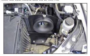
12. Install the heat shield assembly into position so the mounting studs are in the air box mounting grommets.
