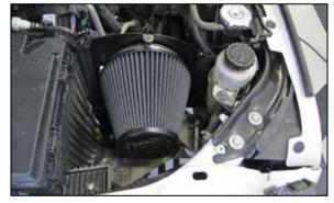
13. Install the AIRAID air filter onto the filter adapter and secure with the provided hose clamp.
