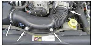
3. Remove the two bolts which secure the factory intake tube to the fan shroud. Loosen the hose clamp securing the factory intake tube to the air filter housing. Loosen the hose clamp securing the factory intake tube to the throttle body.
