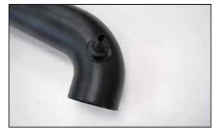
23. Remove the inlet air temperature sensor from the factory intake plenum then install the inlet air temperature sensor into the AIRAID intake tube as shown.
