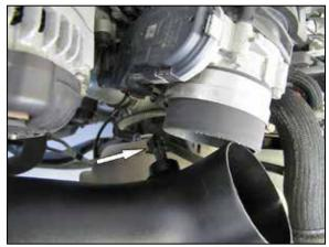
26. Lower the AIRAID tube into place and reconnect the inlet air temperature sensor electrical connection..
