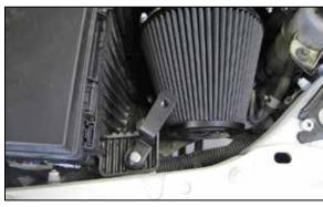
17. Install the provided bracket (083163) onto the rubber mounted stud using the provided hardware.
