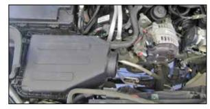
5. Disconnect the crank case vent hose from the crank case vent tube. Lift up and remove the air filter housing from the vehicle.
