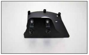
9. Install the two heat shield bracket assemblies onto the heat shield as shown.
