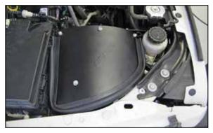
18. Install the AIRAID filter lid and secure with the provided hardware.
