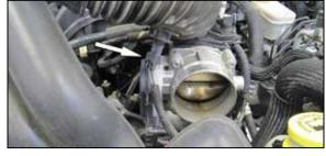
4. Lift up the intake tube and then disconnect the inlet air temperature electrical connection. Then remove the intake tube from the vehicle.
