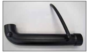
22. Install the provided crank case vent hose onto the fitting as shown.
