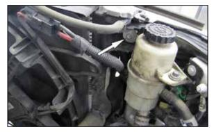
7. Remove the bolt shown that secures the radiator to the core support.
