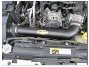
27. Install the AIRAID intake tube into the coupling hose at the filter adapter and then into the hose at the throttle body, then secure with the provided hose clamps.
