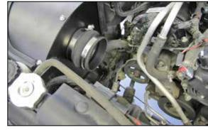
19. Install the provided hump hose (08699) onto the filter adapter and secure with the provided hose clamp.
