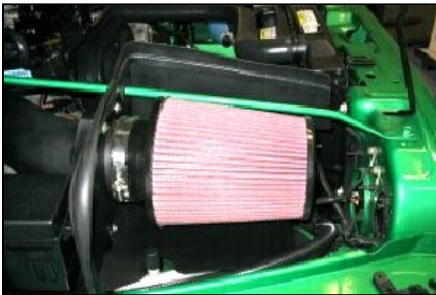
14. Install the Airaid filter on the end of the intake tube. Install the weather strip on the top edge of the Cool Air Dam. (Note: Start at one end and work your way around to insure proper alignment.)
