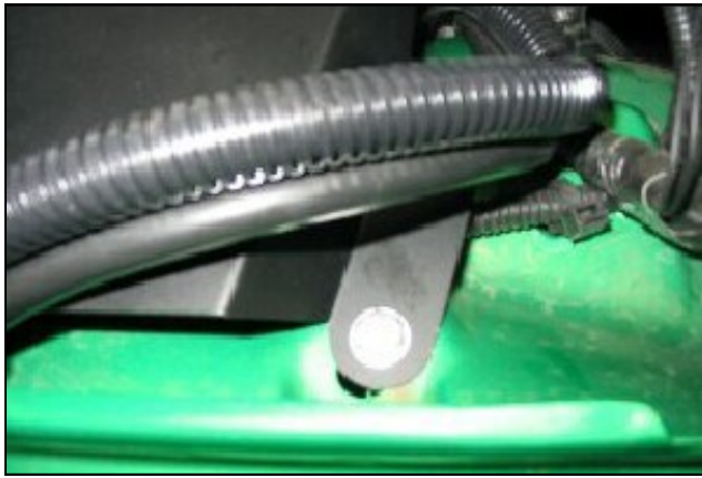
11. Using the supplied hardware and 7/16" socket, fasten the front of the Airaid Cool Air Dam to the fender.
