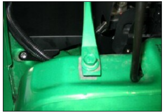
12. Using a 1/2" socket, reinstall the original bolt on the radiator support rod.
