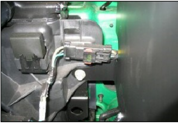
10. Using a 7/16" socket, reinstall the original bolt through the Airaid Cool Air Dam and radiator fan cover.
