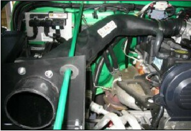
13. Install factory throttle body coupler on end of Airaid intake tube and position assembly on engine as shown. Mount Airaid intake tube to Cool Air Dam using two supplied 1/4"-20 bolts and washers provided. Connect factory breather hose to Airaid intake tube.
