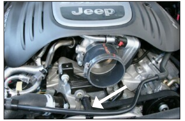
15. Install the coupler and two #60 hose clamps on the throttle body as shown. Do not tighten the clamps at this time. Secure the breather hose to the air conditioner line using the supplied zip tie.
