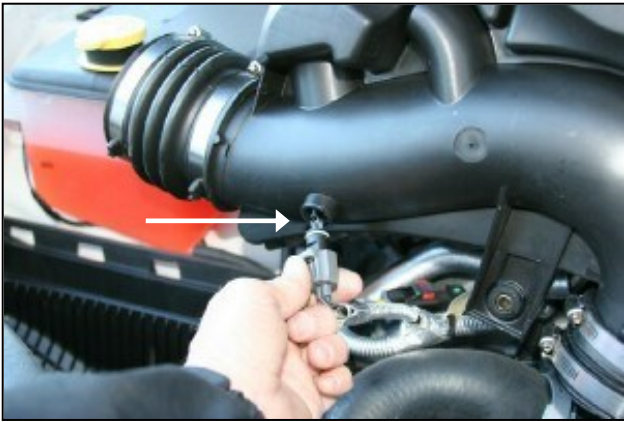
10. Carefully twist and remove the temperature sensor from the bottom of the resonator, and then remove the resonator from the vehicle.
