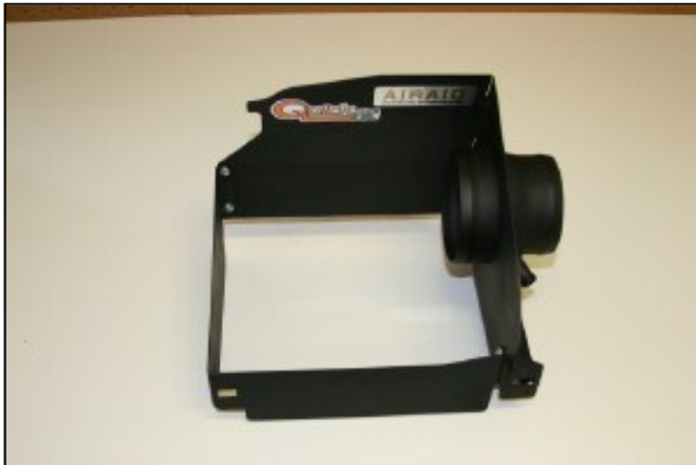
11. Assemble the two pieces of the Quick Fit panels as shown, using the four 6-32 screws, washers, and nuts, that are provided in the kit.
