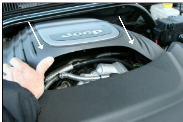
20. Realign the engine cover with the grommets on the engine, and push down firmly to reset the cover.
