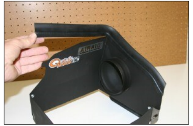
12. Install the weather strip on the top of the Quick Fit assembly. (Hint: start at one end, and go towards the other end, don't start in the middle.)
