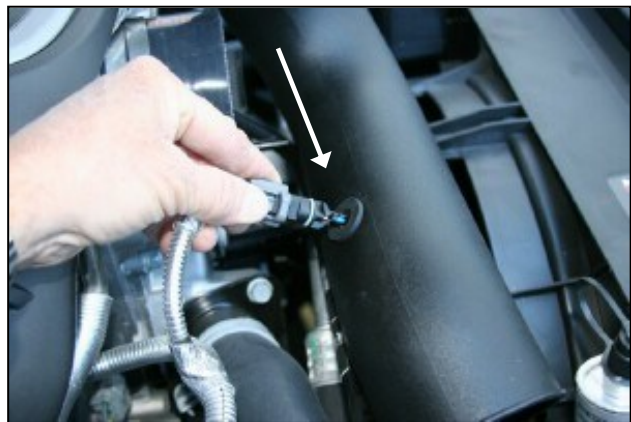
17. Carefully install the temperature sensor into the grommet. Make sure it goes all the way in.
