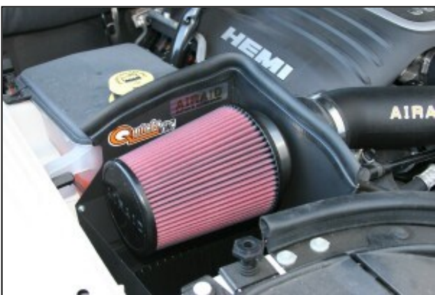
19. Install the Airaid Premium Filter on the Quick Fit assembly as shown, and tighten the hose clamp.
