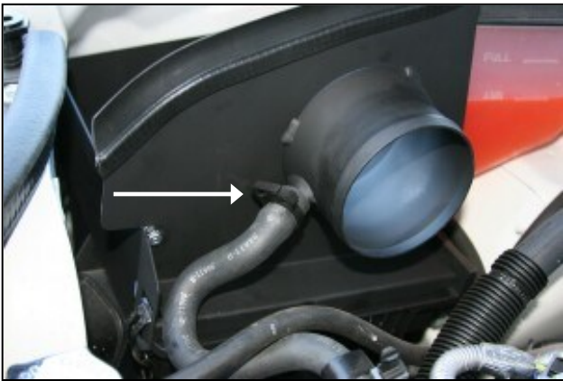
13. Install the Quick Fit assembly in the bottom of the stock air box by sliding the four tabs on the back into the slots on the airbox, once installed, re-hook the two latches. Next, install the speed clamp over the breather hose and connect it to the Quick Fit assembly as shown.
