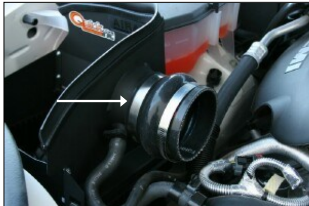
14. Install the hump hose and two #60 hose clamps on the Quick Fit assembly. Do not tighten the clamps at this time.
