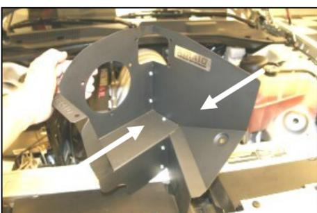
**7.** Assemble the two Cool Air Dam (CAD) panels (#2, #3) using five 6-32 x 5/16" screws (#16), #6 flat washers (#17), and 6-32 keps nuts (#18).
