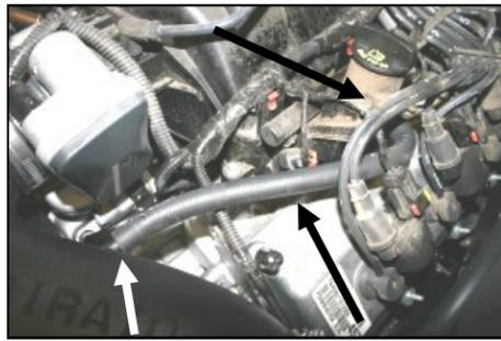
**17.** If you are working on a 6.1L, skip to step #18. If you are working on a 5.7L, install the breather hose (#9) from the valve cover to the Airaid Intake Tube as shown. Re-install the beauty cover onto the engine.
