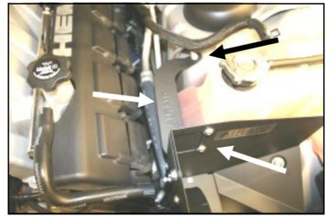
**12.** Install the rear support bracket (#6) from the CAD to the inner fender using three 1/4 - 20 x 1/2" button head bolts (#13), 1/4" flat washers (#14), 1/4" serrated nuts (#15), and the 10mm factory nut removed in step #11.
