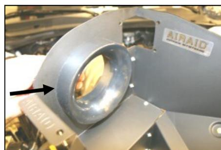
**8.** Next, install the filter adapter (#5) using three 1/4 - 20 x 1/2" button head bolts (#13), and 1/4 flat washers (#14).
