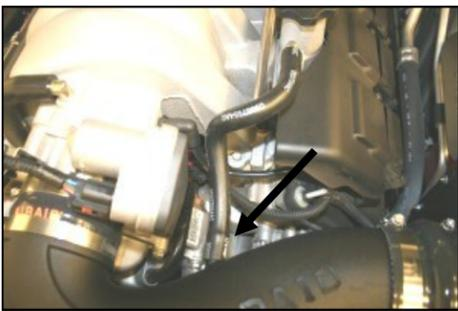
**16.** If you are working on a 5.7L, skip to step #17. If you are working on a 6.1L, reconnect the factory breather tube to the Airaid Intake Tube as shown.
