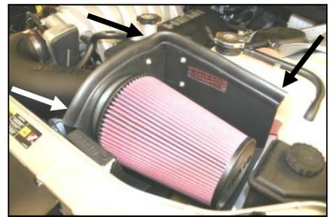
**18.** Install the Airaid Premium Filter (#1), onto the filter adapter inside of the CAD, and tighten the hose clamp. Next install the weather strip (#10) onto the top of the CAD.
