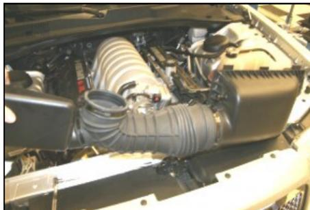
**5.** Remove the factory intake hose and lid assembly from the vehicle. Remove the factory air filter.
