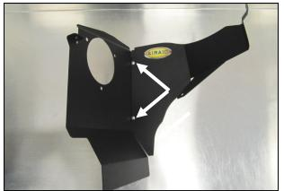
4. Create the panel assembly. Join the Front (#5) and Rear (#6) panels together using the two #6-32 Screws (#18), #6 Flat Washers (#16), and #6 Kep Screws. (#17). Note: The Tab on the Front Panel is to be behind the Rear panel when properly installed.
