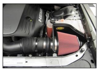
17. Install the Weatherstrip (#8) onto the top edge of the Panels with the contour rolling away from the Filter area. Complete the installation by attaching the Airaid Premium Filter (#1) to the Filter Adapter.
