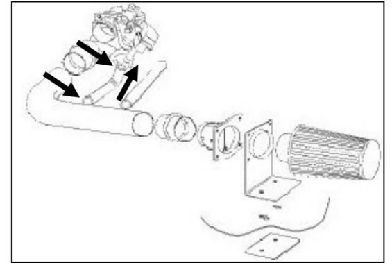
**15. 4.6L engines continued:** Connect the Airaid Intake Tube nipple to the IABV inlet tube using the 3/4 x 1/2" L-hose (#7), and two #22 speed clamps (#17).
