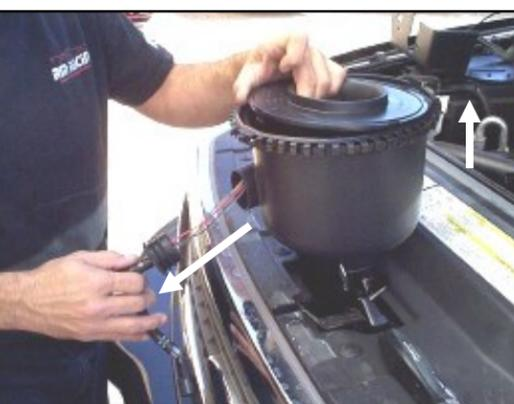
5. The factory airbox assembly is held in place by rubber grommets (it is a "pull to release fit."). Remove the assembly and grommets from the engine compartment. Unlatch the airbox and separate the two sections. Remove the wire loom from the MAF sensor wiring harness, then slide the grommet away from the connector.
