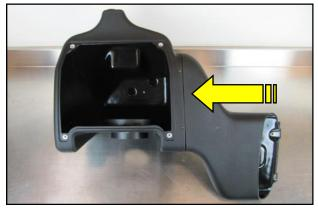
**8.** Snap the new Air Scoop into the Airaid Air Box as
