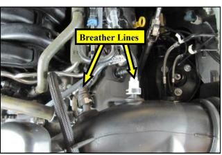
**3.** Disconnect the two breather lines and remove the intake tube from the vehicle.
