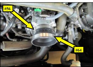
15. Slide the Reducing Coupler and Clamps onto the throttle body as shown. The Small end will use the #56 Clamp and the Large end is to use the #64 Clamp.
