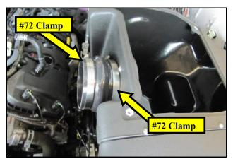
16. Slide the Hump Hose and #72 Clamps onto the Filter adapter, as shown. **NOTE:** On vehicles that were equipped with a wiring
