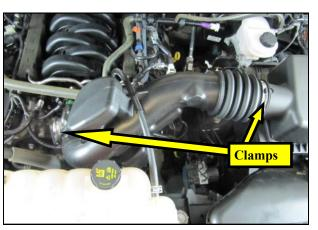
**2.** Loosen the intake clamps on the throttle body and the air box outlet.
