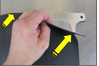
**20.** Remove the protective film from the top of the Air Box Lid.
