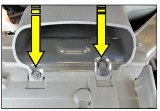
11. Align the mounting holes in the Inlet with the core support holes and secure it using the new, Airaid supplied, Plastic Rivets.
