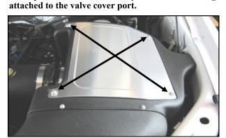
21. Mount the Lid onto the Air Box using the remaining Button Head Screws. Double check your work! Make sure all clamps, hoses, bolts, and screws are tight. Reconnect the negative battery cable!
