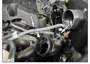
11. Disconnect the green EVAP connector and unhook the line from the retaining clip.
