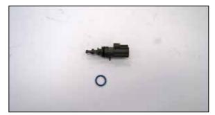
18. Remove the inlet air temperature sensor from the factory air filter housing and then remove the factory O-ring. Install the provided O-ring onto the inlet air temperature sensor.
