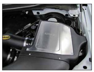
25. Install the air filter housing lid and secure with the provided hardware.
