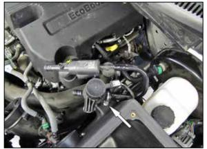
10. Remove the two crank case vent hoses from the solenoid valves and turbo inlet tubes and set aside. Using the provided clamp, secure the solenoid pack to the AIRAID air filter housing. Rotate the brake booster hose where it attaches to the solenoid pack so the it lines up with the brake booster and does not cause a bind.
