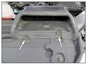
4. Remove the two retaining clips that secure the factory fresh air intake to the core support.
